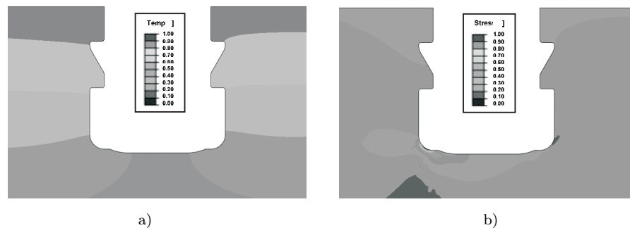
Figure 15: Temperature (a) and equivalent Huber-Mises-Hencky stress (b) distribution in first blade groove after 1500 s from the beginning of start-up.
