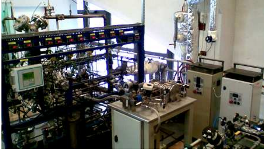
Figure 1: ORC test bench at the laboratory belonging to the Szewalski Institute of Fluid-Flow Machinery PAS in Gdańsk.
