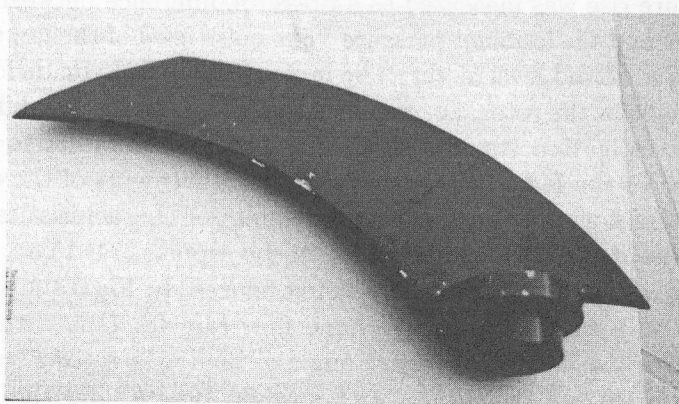
Figure 3. Picture of the swept blade applied in the fan WOO-63 (forward sweep).
