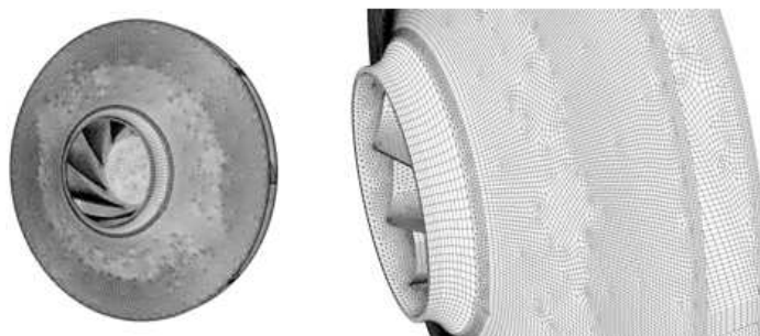
Figure 7. The computational mesh of the impeller surface of the blower aggregate BA0 .
