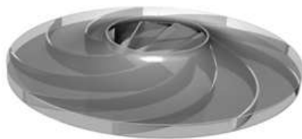
Figure 4. The three-dimensional computational domain of the impeller of the blower aggregate BA0 .
