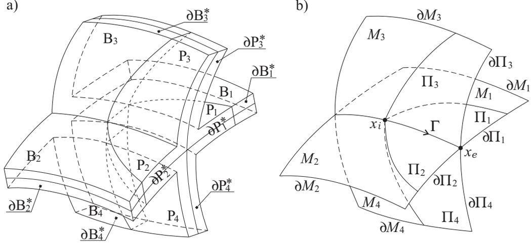
Fig. 4. The self-intersecting shell structure: a) the 3D shell, b) the corresponding 2D base surface.
