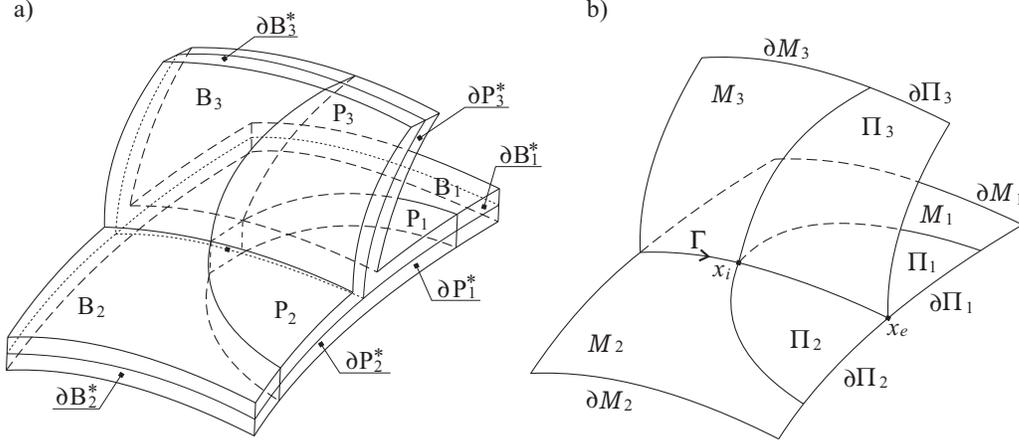
Fig. 2. The branching shell structure: a) the 3D shell, b) the corresponding 2D base surface.
