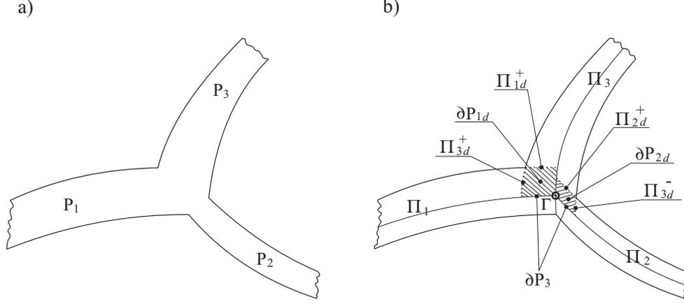
Fig. 6. Cross section of the general branching shell: a) the 3D shell, b) extended strips with fictitious tractions and tubes of double integration.
