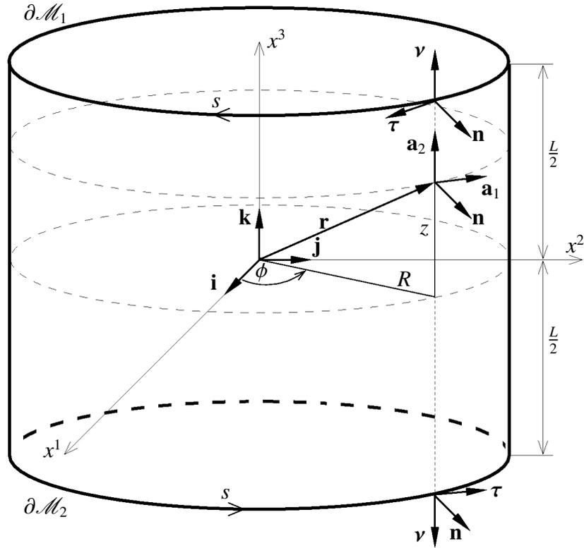
Figure 6: Surface and boundary base vectors on the cylinder.
