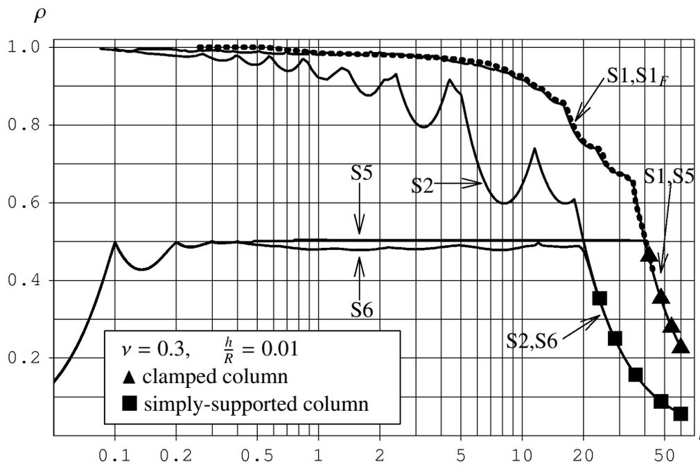
Figure 3: The buckling load of axially compressed perfect cylinder for boundary conditions S1, S2, S5 and S6.
