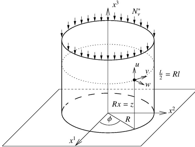
Figure 1: The parameterized upper-half of the cylindrical surface.
