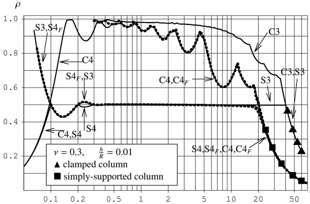
Figure 4: The buckling load of axially compressed perfect cylinder for boundary conditions S3, S4, C3 and C4.
