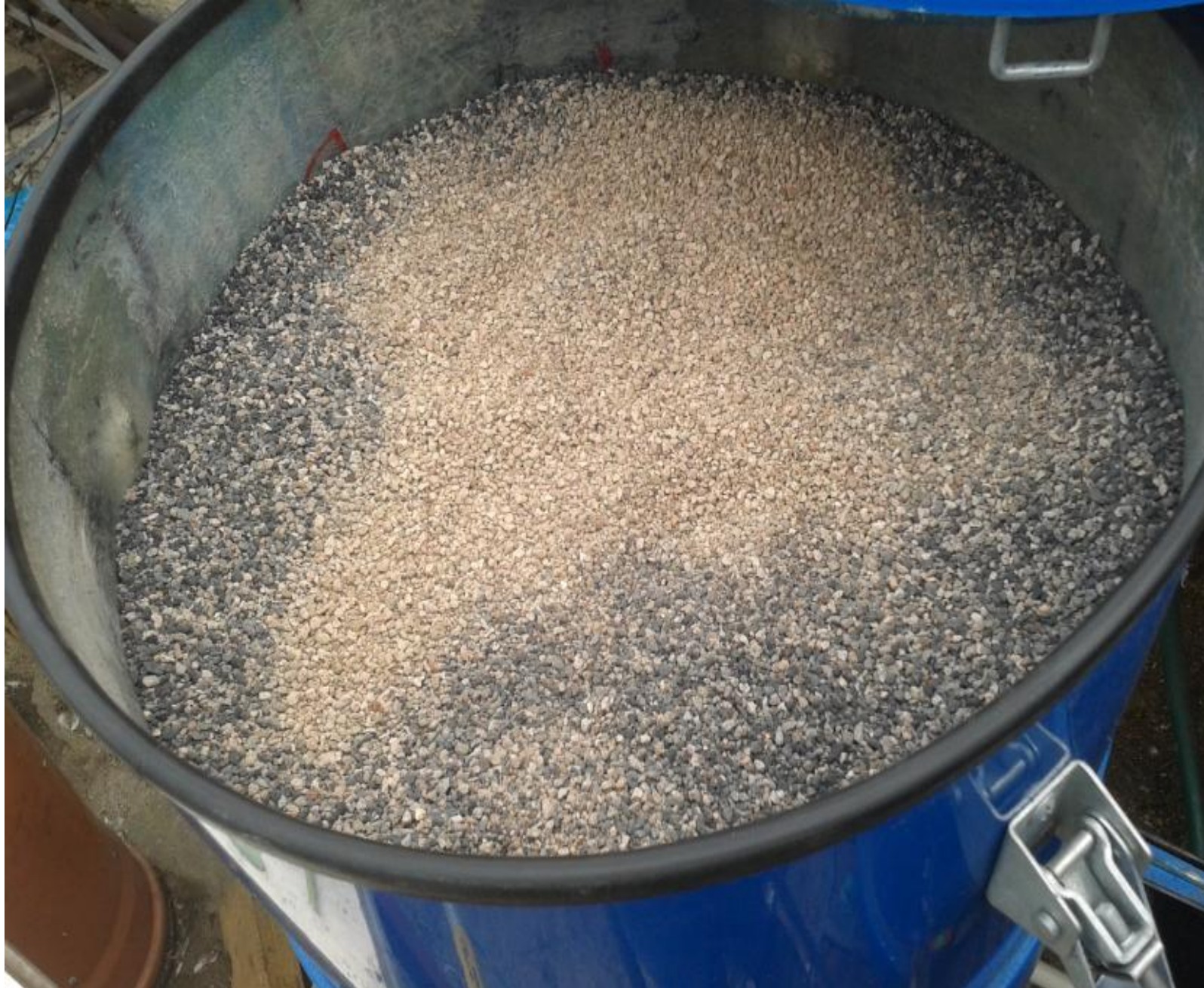
View of sorbent on the IV shelf (outflow ). Privileged places of the flow are visible (darker).
