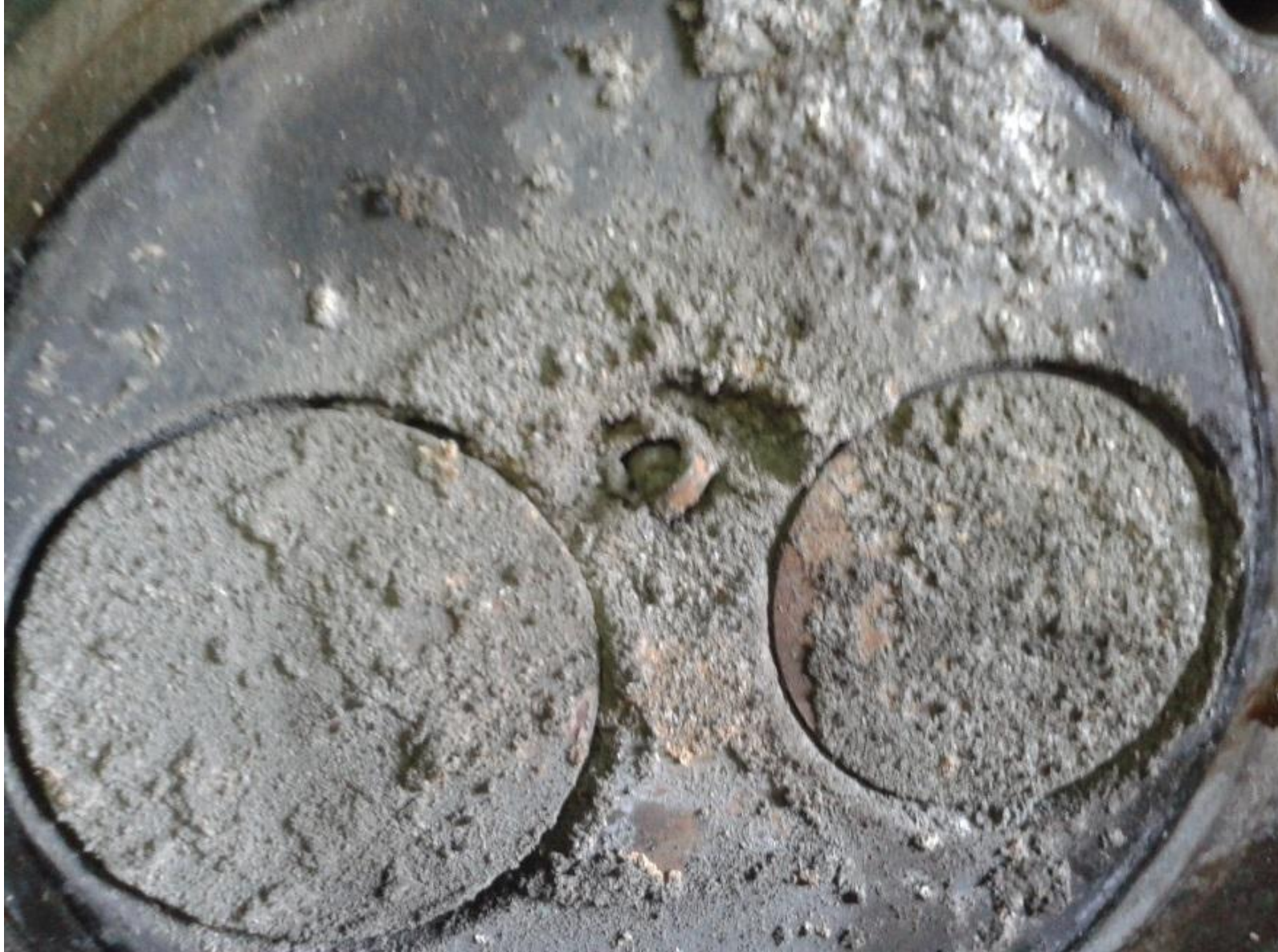
View of carbon deposits on cylinders of the engine burning raw biogas after c 1500 working hours.
