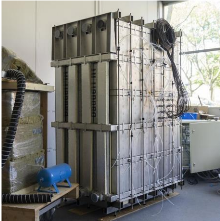
A prototype with "cabinets", each of which is a separate thermal battery module [37].
