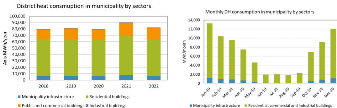
Fig. 3.63. Annual and monthly municipality heat consumption for objects connected to district heat supply by sectors.
