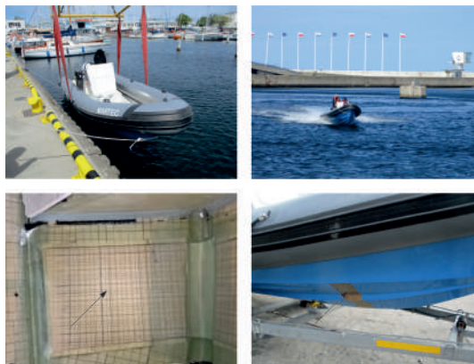
Fig. 3.11: Photographs of fast patrol boat with FBG sensors location area marked by an arrow.
