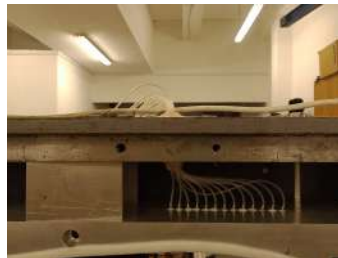
Fig. 13.23: Sealing the tubing leading hole with Play-Dough.
