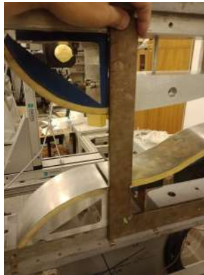
Fig. 13.18: Setting the position of the second inlet element using a straight edge.
