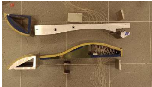
Fig. 13.17: Trial assembly of the nozzle.
