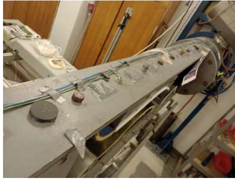
Fig. 13.24: Mounting holes closed and sealed.
