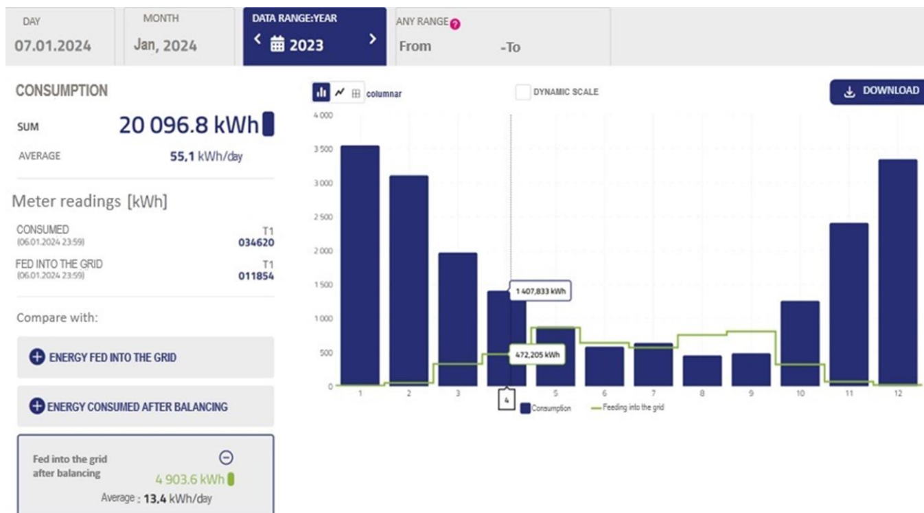
Fig. 8. Visualization from the TAURON e-counter platform. Balance of electricity consumed and energy from the PV installation fed into the power grid - considering the settlement balance [23].
