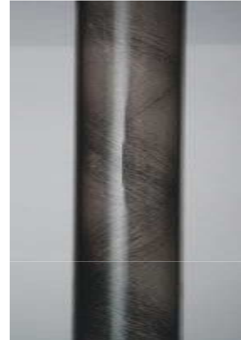
Visualization of the swirl: the discharge quartz tube covered with the soot after plasma processing of ethanol
