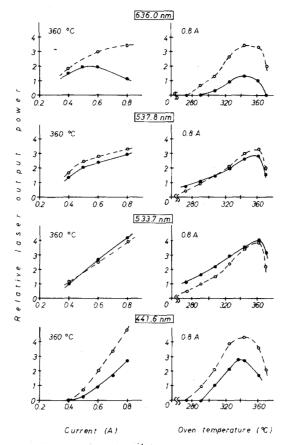
Fig. 4. The dependence of He-Cd<sup>+</sup> laser power on the discharge current and oven temperature for the longitudinal (broken line) and transverse HCD. Simultaneous multiline operation. Helium pressure 16, 4 mbar.
