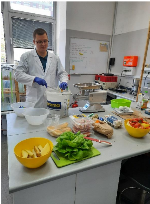
Photo 3. Preparation of model organic waste for production of organic fertilizer
