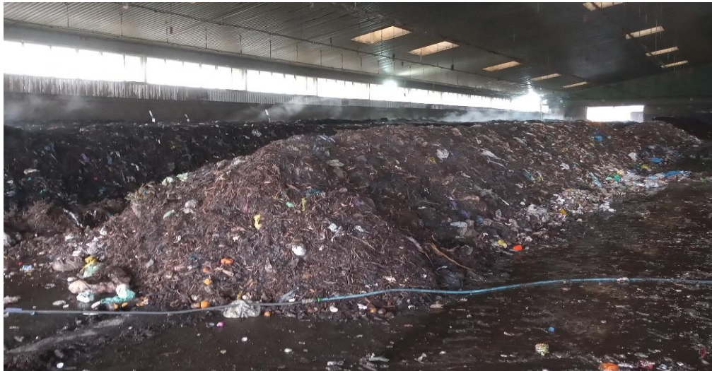
Fig. 5 Composting pile of source sorted fraction of municipal solid wastes
