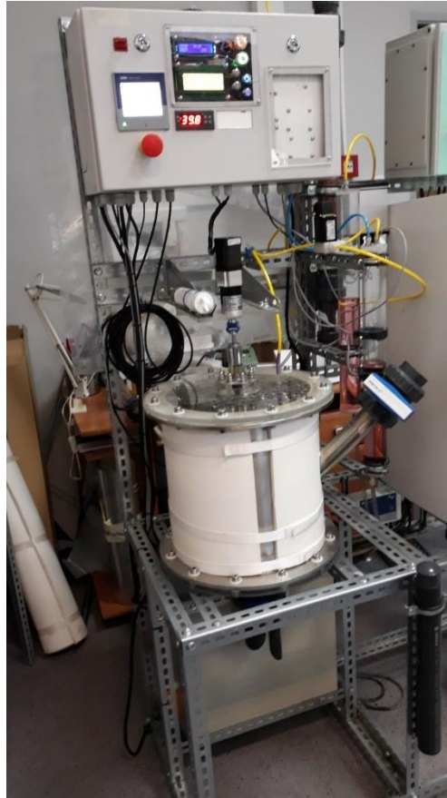
Fig. 18 Reactor for semi-continuous fermentation
