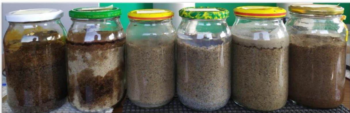
Fig. 1. Visual effect of waste-based stabilizers affecting the soil sealing influencing its frost resistance
