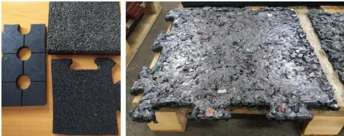
Fig. 2. Products from waste tires (left) and PLASTRY Kuligowskiego® (right)
