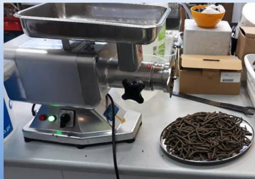
Pre-drying and pelleting
