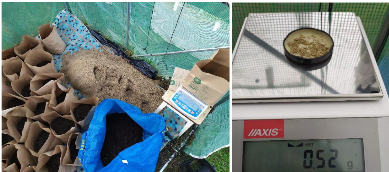
Figure. 5 Soil preparation by mixing the pre-sieved sand with peat (5:1 w/w) – left and grass seeds weighing – right.
