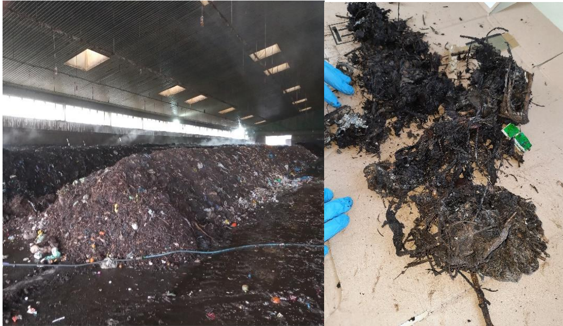
Photo 2. The prism treated with EM (left) and Preliminary separation of rocks and glass before grinding the compost sample (right)
