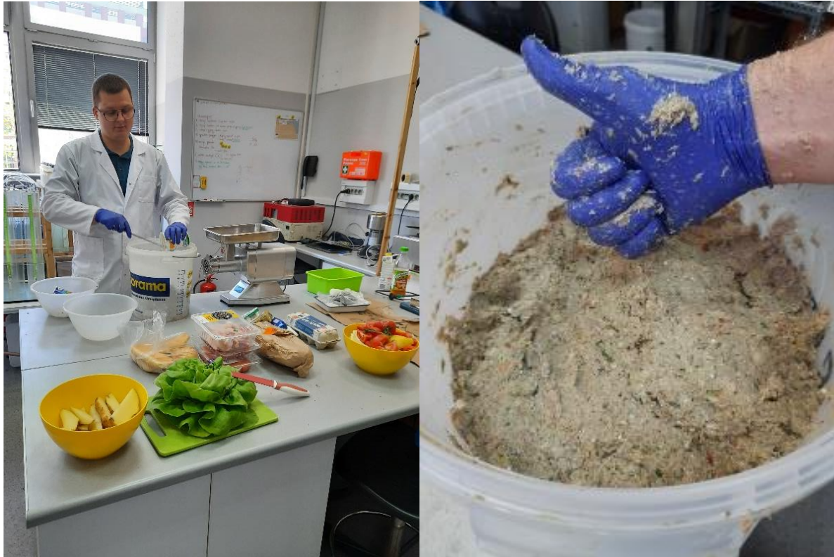
Photo 3. Preparation of model organic waste for production of organic fertilizer (left) and waste before methane fermentation (right)
